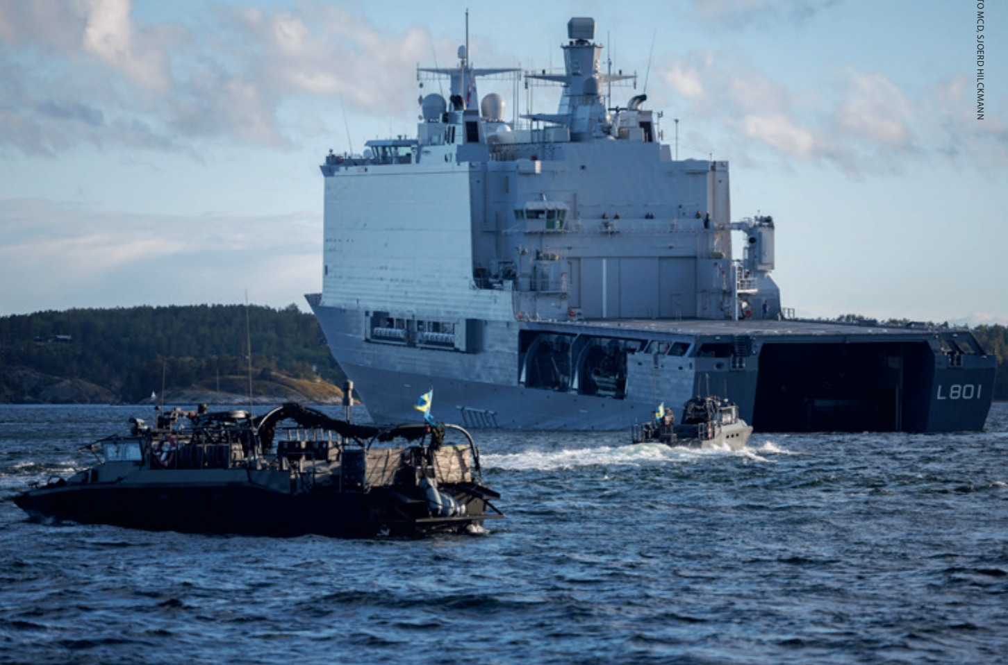
HNLMS Johan de Witt participated in Exercise Baltops24. During the exercise, the ship experienced loss of GPS for a specific duration as a result of solar radio bursts. System redundancy mitigated the effects: the ship's inertial navigation system was more than accurate enough to bridge that timeframe
