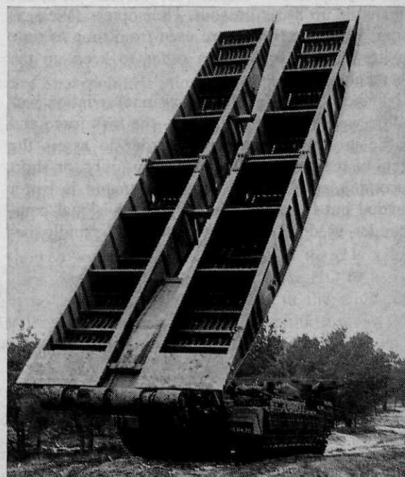
A tank mounted bridge on a Centurion chassis, able to cross gaps up to 13.7 m, can be laid in three minutes
