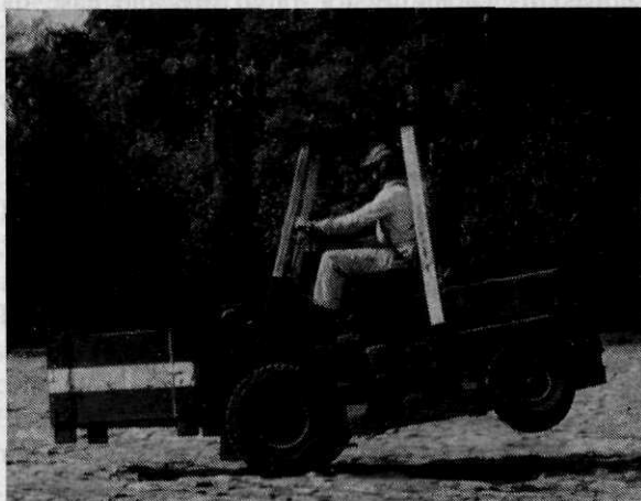
Fig. 3 Lansing Bagnall FODR 6 fork truck, designed primarily for fast, heavy duty outdoor operations, undergoing rigorous tests
