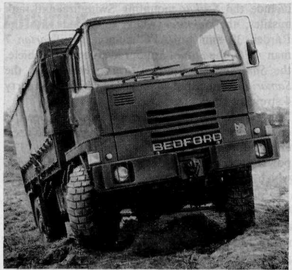
Fig. 1 Prototype Bedford TM 4-4 four wheel drive 'go anywhere' truck for 8 tons payload class
