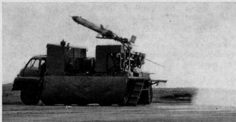
AN/USD/501 Reconnaissance Drone Midge , a drone which the British Army uses to carry a camera over enemy territory to photograph enemy activity; it flies a pattern which has been programmed before launch, and returns to a pre-determined spot where its engine cuts and its parachutes open to bring it gently to the ground. Midge is operated by the Royal Artillery
