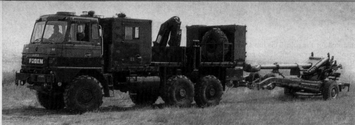
The new British light gun 105 mm with its trails reversed being towed by the Foden Artillery tractor
