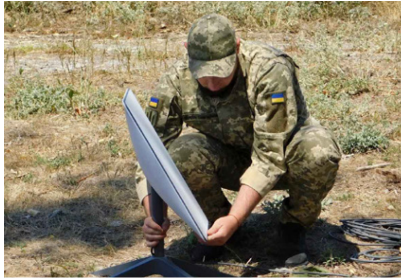
A Ukrainian soldier installs a Starlink internet terminal. Access to the Starlink satellite network mitigated the effects of Russia's attack against Ukrainian satellite communications
